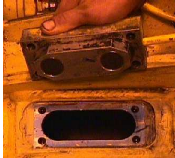
Figure 5 – Magnetic proximity switches installed in the upper-cylinder of a modern diesel hammer
