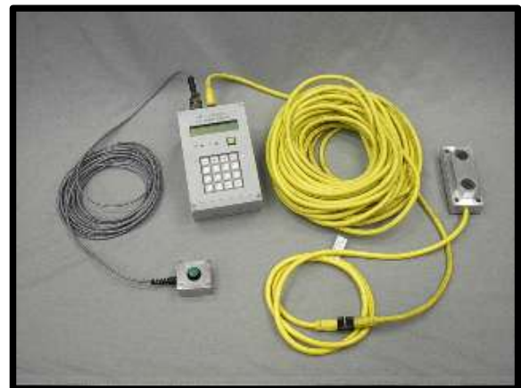
Figure 7 – Pile Driving Monitor from 2002
