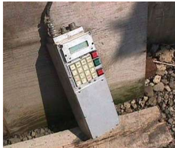
Figure 6 – Pile Driving Monitor from 1990
