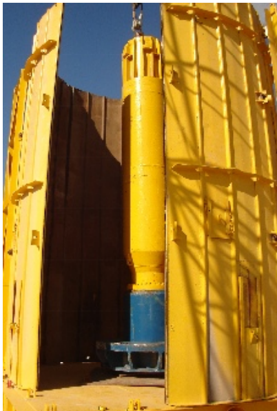
Newly upgraded 40 MN STATNAMIC device during onsite assembly.
