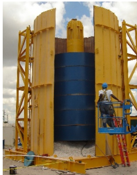
Newly upgraded 40 MN STATNAMIC device during onsite assembly.
